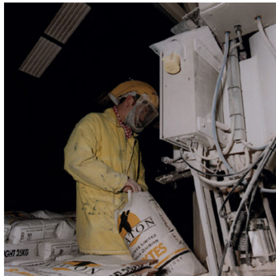
Figure 5a Bagging operation in a mineral processing plant: under ambient light and with flash, dust cloud is not visible
