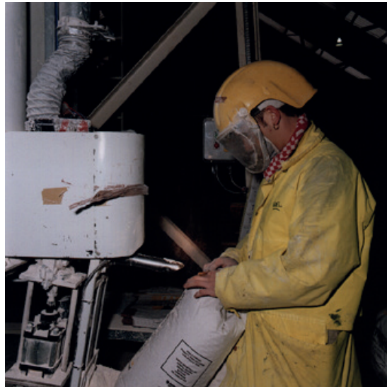
Figure 5c View from the same side of the lamp and with flash: dust cloud is not visible
